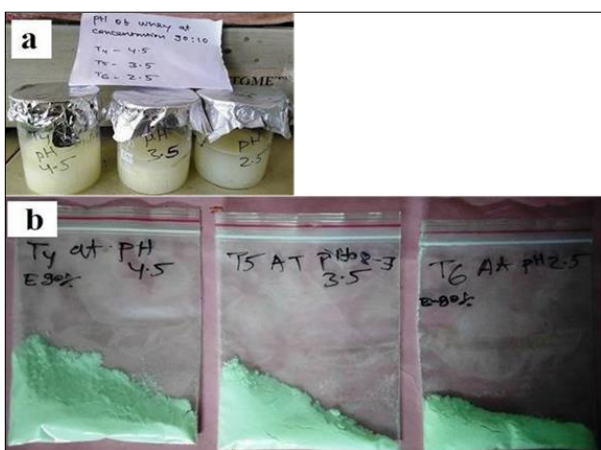
Fig 4: pH adjusted paneer whey treated with solvents for extraction of lactose. (a) Before crystallization and (b) Final Product
