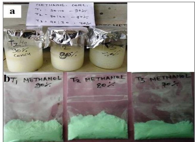
Fig 5: Paneer whey treated with methanol for extraction of lactose. (a) Before crystallization and (b) Final product
