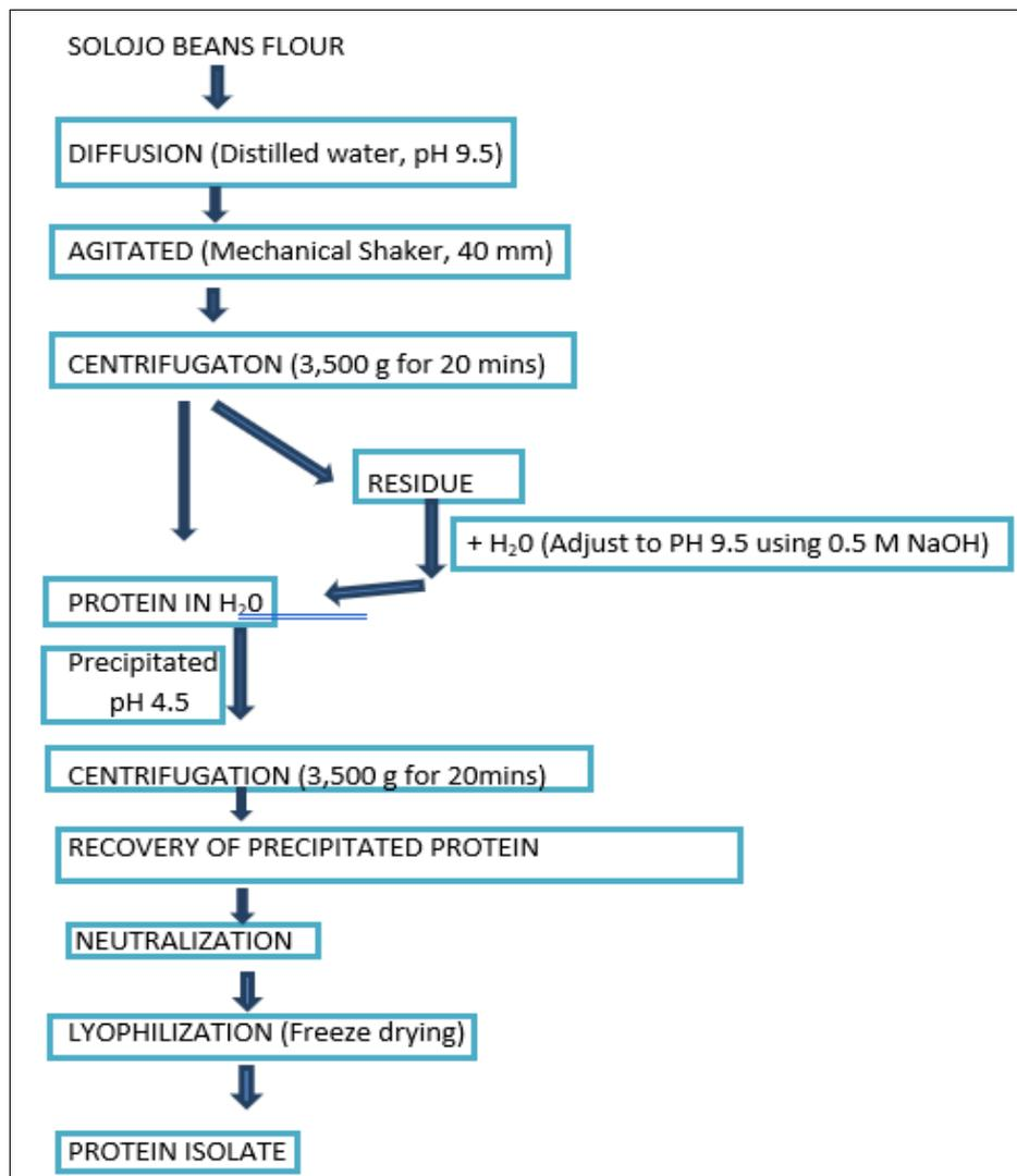
**Fig 6:** Schematic diagram for the processing of protein isolate (Adebowale *et al.*, 2007modified)
