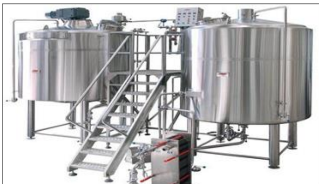
Fig 2: Orange jelly drinks syrup preparation and cooking tank
