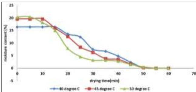
**Fig 3:** Effect of drying temperature on the moisture content of green peas in food dehydrator
