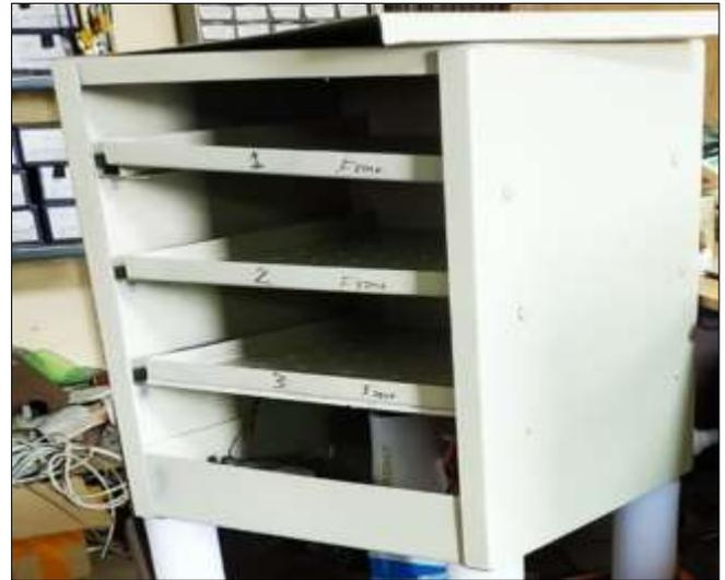
**Fig 2:** Portable food dehydrator equipment
