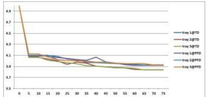
**Fig 5:** Effect of tray position on green peas drying time at 50°C at portable food dehydrator (PFD) and tray dryer (TD)
