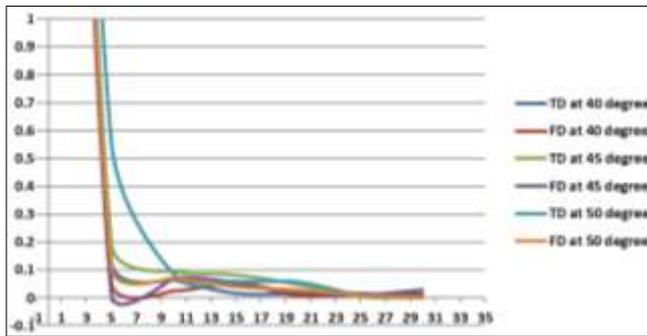
Fig 7: Effect of drying principle on green peas drying rate at 40°C, 45°C & 50°C
