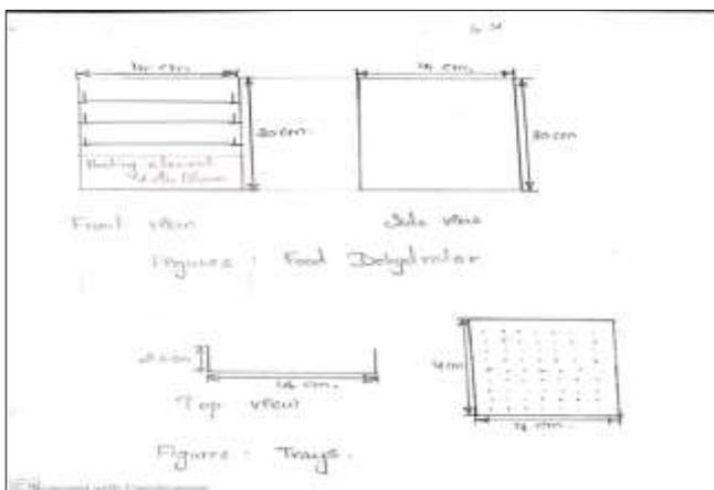
**Fig 1:** Design of portable food dehydrator
