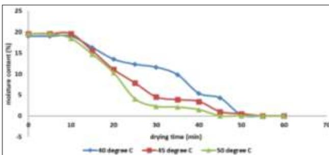
**Fig 4:** Effect of drying temperature on the moisture content of green peas in tray dryer
