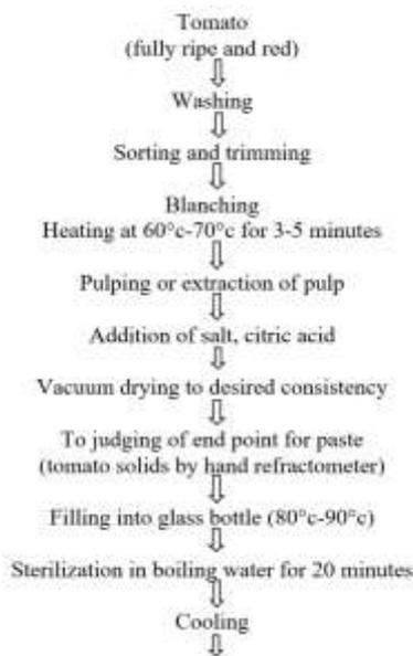
Fig 1: flow diagram for production of tomato paste
