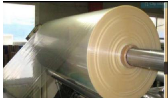
Fig 4: Nano-Silica coated high oxygen Barrier Nylon (OPA) Films for food packaging
