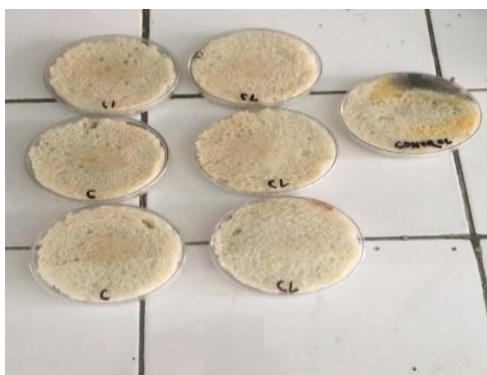
Fig 3: Samples in contact with film (Observation as on 8th day) *C-Cinnamon film, CL-Clove film, Control film
