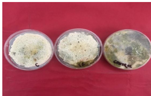
Fig 4: Samples in contact with film (Observation as on 9th day) *C-Cinnamon film, CL-Clove film, Control film
