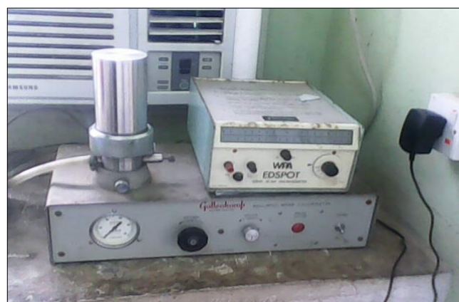
Fig 1: Gross Energy Determination Using Gallenkamp Ballistic Bomb Calorimeter
