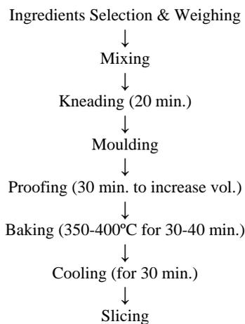
Fig 1: Bread making flow process
