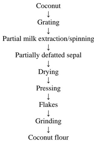
Fig 1(a): Flow chart for the production of coconut flour
