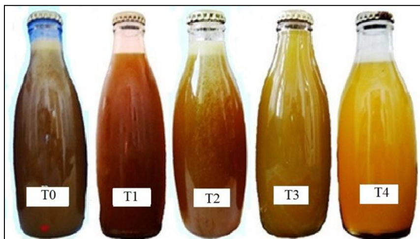
Fig 1: Photograph of liquid jaggery packed in glass bottle prepared by different treatments; T0= Control, T1= Juice clarified through muslin cloth, T2= Juice clarified by sodium hydroxide (NaOH), T3= Juice clarified by centrifuge, T4= Juice clarified by membrane filtration
