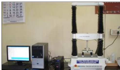
Plate 1a: Analysis of texture using Texture analyser
