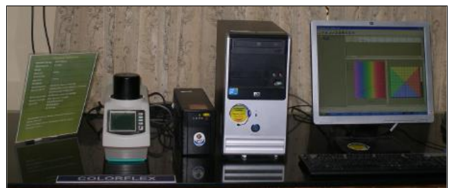
Plate 2: Analysis of colour using Hunterlab colourflex
