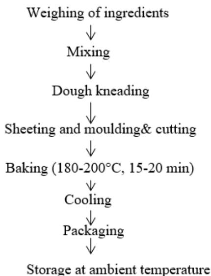
Fig 3: Flow chart for production of biscuits
